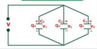
The Voltage across each capacitor is the same, and it is equal to the voltage of the battery.
