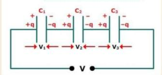
Charge stored on each capacitor is same and equal to the magnitude of the charge, which comes from the battery...
